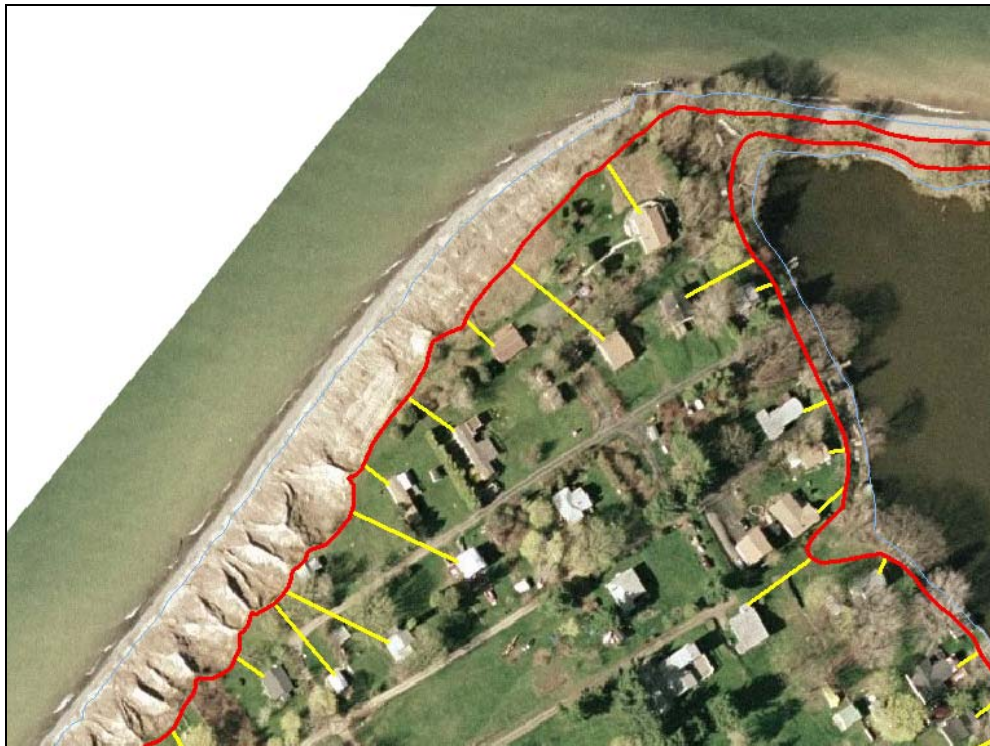
Figure 2 - Example of Bluff Distance Mapping, CND7 (Top) and US4 (Bottom)
